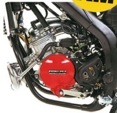
The Yamaha Minarelli 50cc, two-stroke, liquid-cooled engine.
